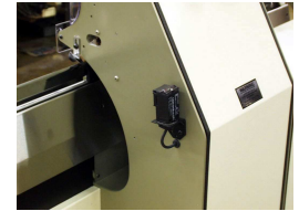
Missing book sensor on 201CB Models eliminates dropped stitches that can jam and break clinchers
