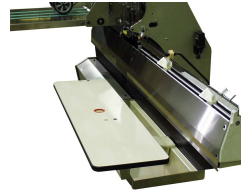
Two-station saddle provides four times greater productivity than pedestal stitchers.
