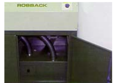
Optional fume/chip exhaust collects binding byproducts.
