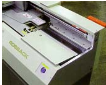
Optional auto-nipping offers the most significant production time savings, while providing a square, tight book.
