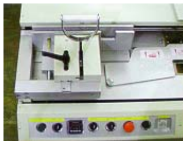
Optional auto-clamp reduces initial setup time. Optional vibrating clamp jogger minimized any sheet edge irregularities.
