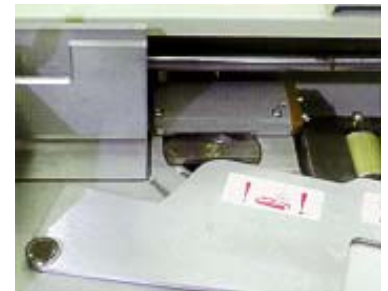
Optional milling smooths paper edge irregularities and allows you to bind complete signatures.
