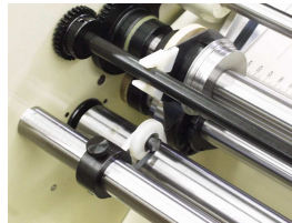
Sturdy nylon burr flatteners are easily adjusted over perf lines eliminating build-up for re-feeding through presses, collators and all other automatic equipment, plus the added benefit of easy jogging.
