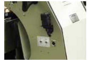
Sensor detects missing signatures over saddle and prevents stitching heads to stitch without a book present.
