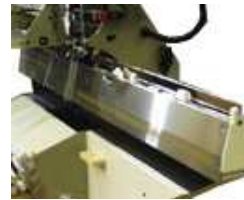
Two-station saddle & feed fingers provide 4x greater productivity compared to pedestal stitchers.
