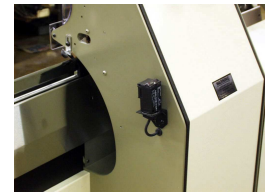
Sensor on 201B Models detect missing signatures over saddle and prevents the stitching heads to stitch without a book present.
